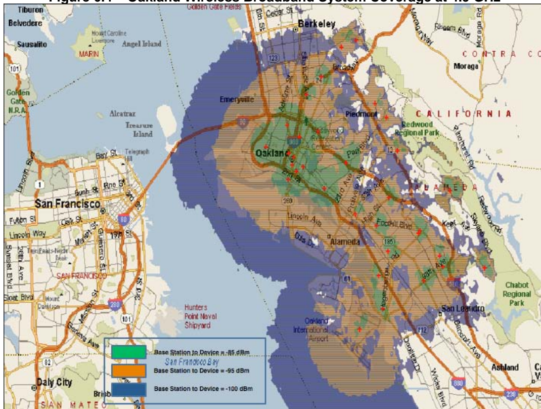
Figure 6.4 – Oakland Wireless Broadband System Coverage at 4.9 GHz
